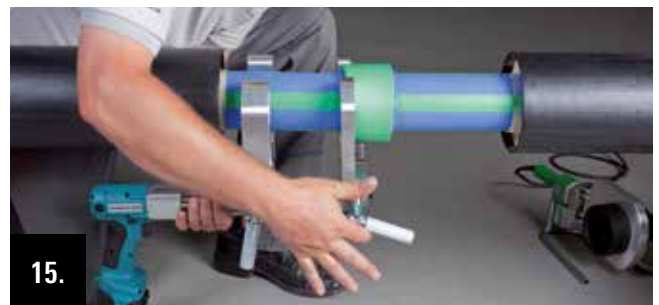
Release the clamping jaws on the fitting side by unscrewing the fixing jaw.
