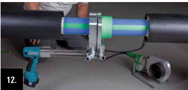
Align the welding connection with the welding jig and fix it shortly. The further processing is proceeded after the specified cooling time.
